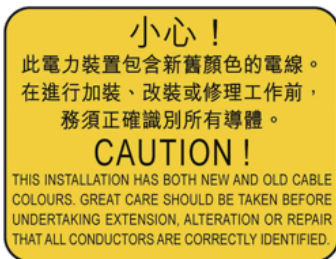
Figure A18(3) - Warning Notice
